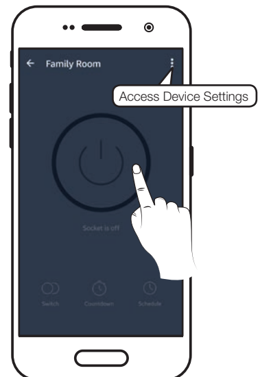
THIS IS THE CONTROL SCREEN. HERE YOU CAN TURN THE PLUG ON, SET TIMERS AND SCHEDULES, AND ADJUST SETTINGS.
