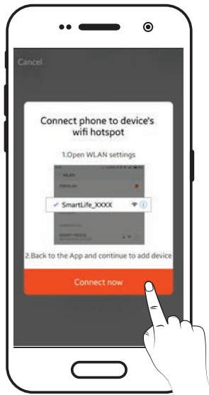
SELECT CONNECT NOW TO PROCEED TO YOUR ANDROID PHONE'S WI-FI SETTINGS MENU. APPLE IOS USERS, EXIT THE APP AND MANUALLY ACCESS YOUR WI-FI SETTINGS MENU.
