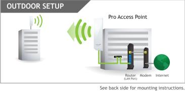
Connect the Pro Access Point to your Router or Network Switch
