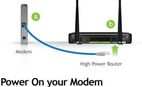
Connect the other end of the cable to the blue Modem port on the High Power Router.
